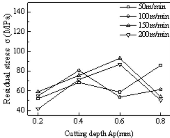
Fig. 6. Cutting speed - cutting depth on the influence of residual stress ( $f=0.04\text{mm/z}$ ,  $A_e=8\text{mm}$ )
