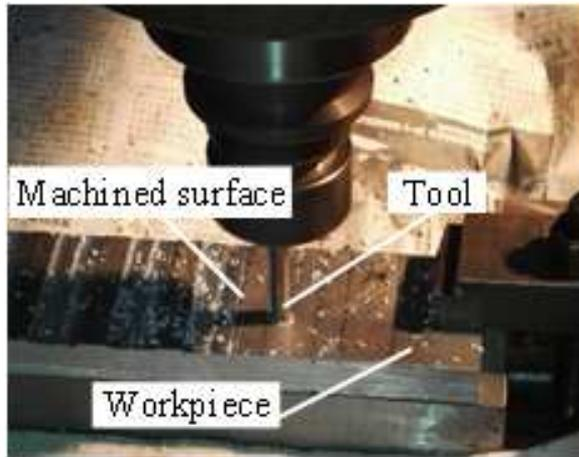
Fig. 2. The milling test scene
