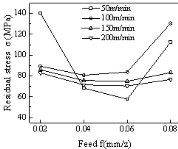
Fig. 5. Cutting speed - feed on the influence of surface residual stress ( $A_p=0.4$ mm,  $A_e=8$ mm)
